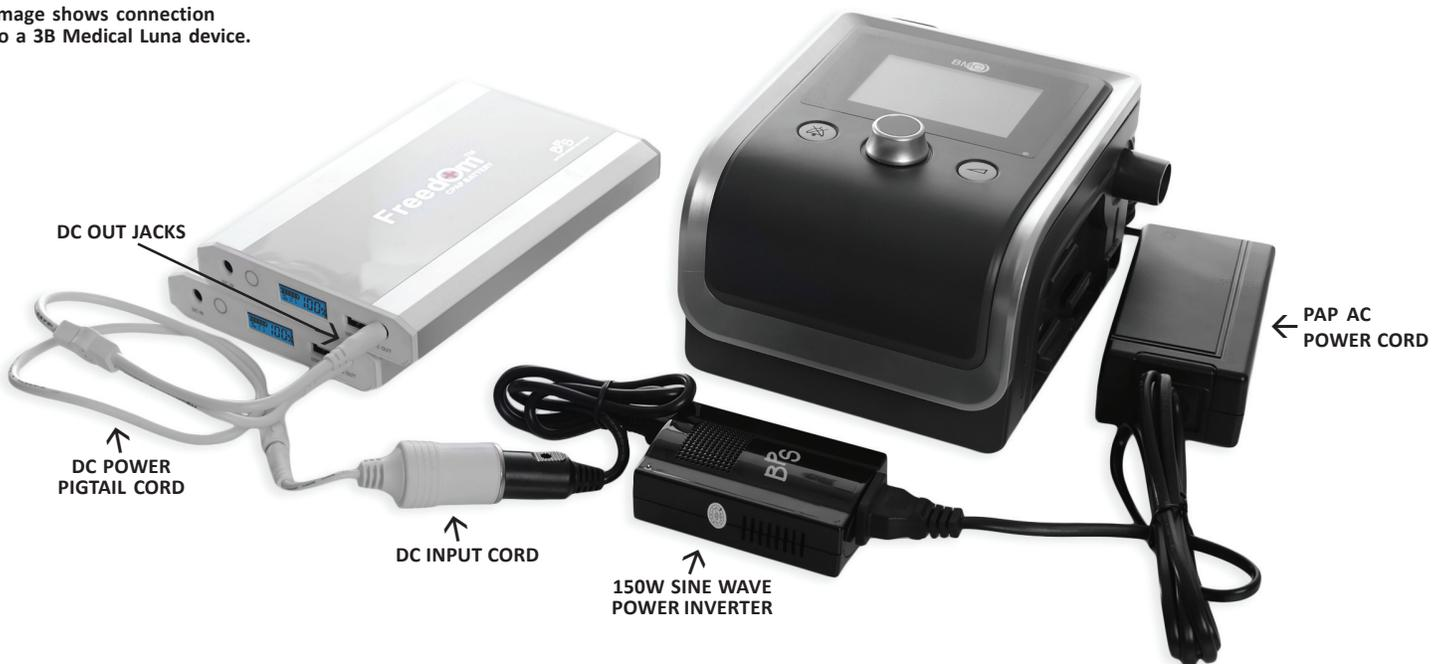
The inverter can also be used to charge the battery in a vehicle (vehicle does not need to be running) and to power/charge other small electronic devices with the battery. The inverter is not proprietary to the Freedom™ CPAP Battery and can be used with other external batteries.
