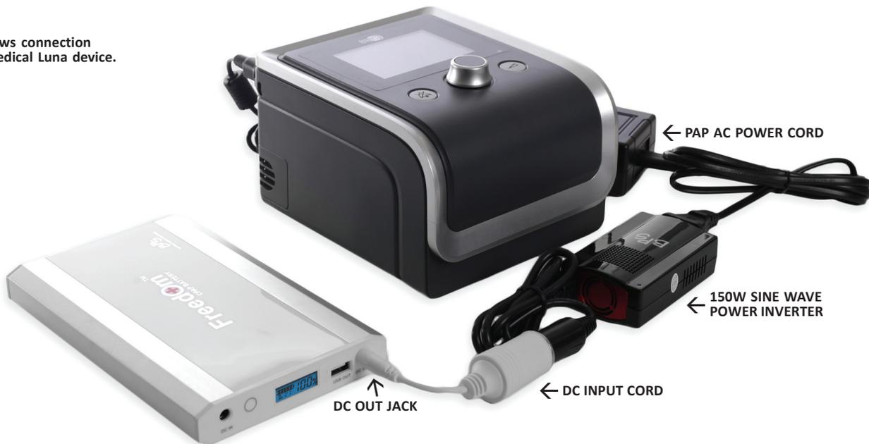
The inverter can also be used to charge the battery in a vehicle (vehicle does not need to be running) and to power/charge other small electronic devices with the battery. The inverter is not proprietary to the Freedom™ CPAP Battery and can be used with other external batteries.
