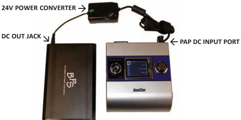
**Note:** ResMed's S9 Series DC/DC Converter or a sine wave power inverter may also be used to complete the connection between the ResMed S9 device and the Battery Pack.
