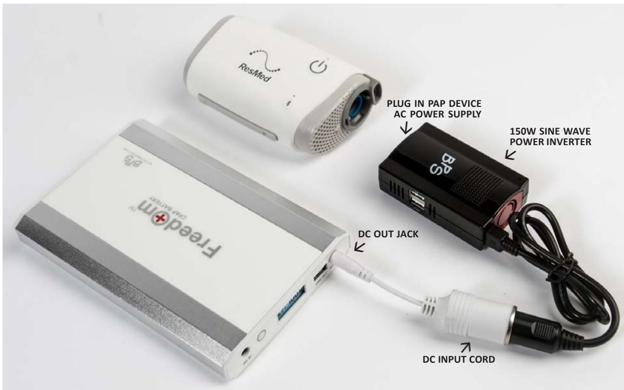
The inverter can also be used to charge the battery in a vehicle (vehicle does not need to be running) and to power/charge other small electronic devices with the battery. The inverter is not proprietary to the Freedom™ CPAP Battery and can be used with other external batteries.
